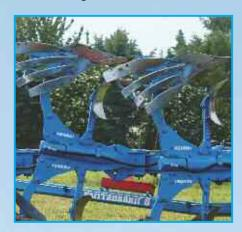
When simultaneously tripping sideways and upwards, normal overload safety devices, based on a fourpoint connection, make the position of the whole plough body unstable as it lifts from three connection points and is drawn back by the mechanical or hydraulic pull element via only one point.
