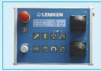
The operator selects the weight transfer to the tractor by choosing and setting a top link operating pressure. A constant oil flow, via one of the tractor spool valves, allows the operating system to monitor and constantly adjust the top link to maintain the selected pressure, and transfer the optimum amount of weight to the tractor.
