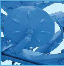
The plain 500mm diameter disc coulters feature side mouldings to provide a positive drive even when cutting through a lot of organic material. Depth adjustment is through vertical swivelling of each coulter arm which is screw-locked into a toothed bracket. The adjustable bearings, fitted with plain side towards the ploughed land, are double sealed against dirt ingress.
