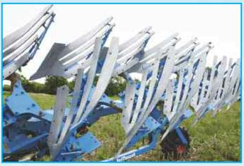
The headland management system optimises weight transfer during headland turns. It transfers some weight to the ploughs land-wheel to ensure the tractor linkage is not overloaded, but leaves enough weight on the tractor to maintain stability when working on hillsides. This fully automatic system creates a safe and efficient working situation for the driver.
