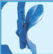
Fitting the skimmer onto a flat stalk avoids the risk of twisting. All shares and mouldboard variants can be exchanged without any problem because the frog is the common to all skimmer types. For ploughing without skimmers, loosening of two bolts allows compete removal of the skimmer arm.
