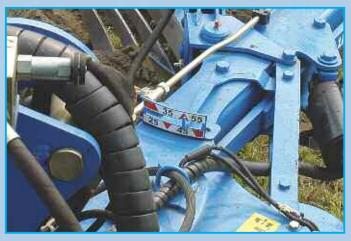
The VariTansanit is equipped as standard with hydraulic working width adjustment from 25 to 55cm per body. The plough can always be set to the optimum working width for the soil, subsequent crop, and situation. Optiquick ensures that ploughing without side draft is guaranteed whatever the working width.
