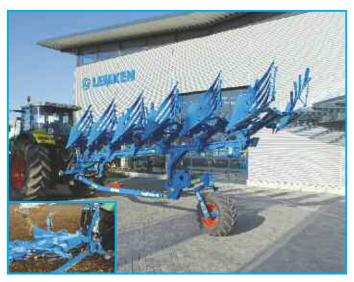
During road transport, the rear wheel is locked, with the plough following the tractor like a trailer. In the field, the headstock pivot is locked, and the land wheel set to its caster position.
