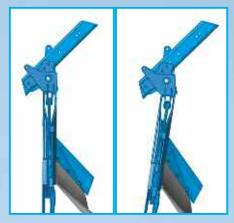
With up to 38cm upward and 20cm sideward movement, there is sufficient tripping capacity to provide continuous trouble free work even when ploughing deep. High trip forces, which are adjustable from the tractor seat, ensure the Hydromatic auto-reset system is always set to combine quality ploughing with efficient plough protection. A further benefit of the system is the lack of lubrication points – the system is maintenance-free.
