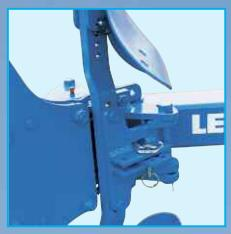
Both the VariTansanit (shearbolt) and VariTansanit T (auto-reset) are available as an option with individual quick adjustment system for the skimmer angle. This allows further fine-tuning of the skimmer performance where required.
