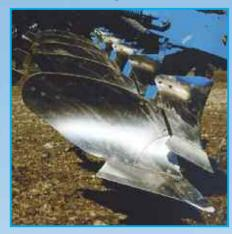
The LEMKEN Dural body is the standard body for LEMKEN ploughs. The frog is hardened and tempered making it immensely strong. The plough body is adjustable for pitch to help soil penetration. The smooth transition from share to mouldboard and the low-resistance profile ensure that the draft requirement of the plough body is minimised.
