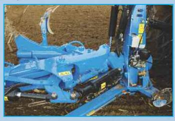
The VariTansanit is equipped with hydraulic frame swivelling, as standard, with an adjustable stop to set front furrow width. The Optiquick turnbuckle allows simple adjustment of the tractor/plough alignment using the spanner provided.
