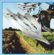
The slats are of thick, completely hardened, special steel and individually exchangeable.
