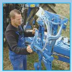
Mouldboards, slats and shins can be exchanged without tools and thus considerably faster than parts from conventional bodies. Simply removing a clip pin, allows the shin to be removed which, itself, acts as a locking device for the slats or solid mouldboard. The point is fixed with a single screw which additionally decreases the replacement time required. Measurements have resulted in set-up times that are 80% lower than that conventional plough bodies.
