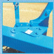
The EuroTitan adjustment brackets are bolted solidly to the frame giving great strength and reliable solidity with a high standard of precision. Loosening the central bolt and withdrawing the positioning bolt allows four different working widths to be selected from, a rapid and simple operation. Other equipment such as skimmers or disc coulters are automatically adjusted at the same time.
