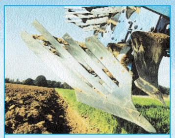
The shares comprise separate component plates of micro-alloy boron-steel. Overlapping design avoids roots or other foreign objects being caught. Tight fitting and firm attachment guarantees, wear resistance and reliability against breakage.
