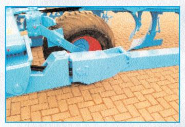
Horizontal pull point can be raised just by moving a bolt, allowing precise weight transfer to the rear axle of the tractor. With a crawler the pull point is fixed very low for equal loading of the tracks. This means that for all types of tractor optimum tractive force transfer is achievable with the associated minimum wheel or track slip.
