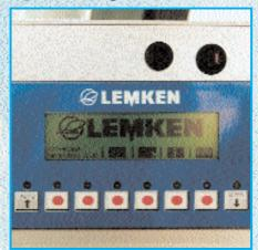
As standard the Titan ploughs are equipped with the electrical turnover control. With this device, the turning and lifting functions is contolled by means of two sensors. The electronic plough control which is available as an option, helps the farmer considerably with its optimal headland management system.
