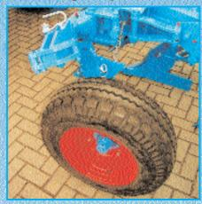
The exact setting of ploughing depth can be finely tuned without tools at the wheel axle as well as by moving the appropriate pin at the rear support wheel. When the plough is set into the ground the rear support wheel is brought automatically into working position thus making impossible an undesirable forward-swinging of the wheel on uneven ground.
