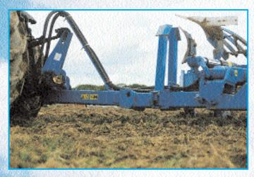
The one-piece shock-absorbing category III or IV plough drawbar is simply adjustable for height. It protects tractor and plough headstock through absorbing larger shock loads. The headstock axle material is well-tempered. The axle runs on roller bearings and is easily lubricated. All this means great strength and long working life.
