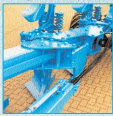
The robust square-tube frame of micro-alloy fine-grained 10 mm steel is notable for its light weight, superior strength and long working life. The frame plates for the mounting of the adjustment brackets are bolted to the frame giving exact precision and long-term solidity.
