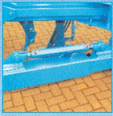
During in-furrow ploughing, front furrow width is adjusted via spindle. The same spindle can be used during on-land ploughing to alter tractor-furrow distance.
