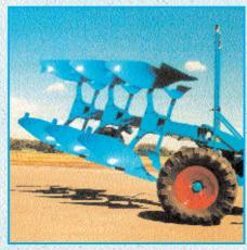
As well as allowing very good adjustment to the contours of the field surface and enabling the front frame to follow downward slopes first, the joint between the plough frames also enables separate raising of the rear plough frame through the electronic plough control. This allows, for instance, the ploughing in one direction with 12 furrows and in the other with eight. The support wheel (10,8/80-12) serves for depth guidance of the rear plough frame.
