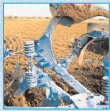
The skimmers of the Titan with automatic overload security system can be adjusted on the beams. Adjustment of working depth is with pins with no tools required. If an adjustment of the throw angle is desired, round legs can be fitted which are secured in the attachment by bolt.
